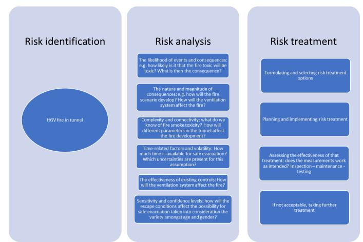
Figure 2: Risk assessment process for fire in a HGV in tunnel illustrated with the ISO 31000 [2] model
