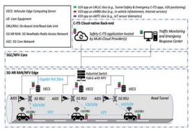
Fig. 2. 5G-based ultra-reliable and low latency network architecture model for tunnel safety communication.
