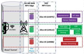
Fig. 1. A sample 5G network slicing model for C-ITS tunnel safety.
