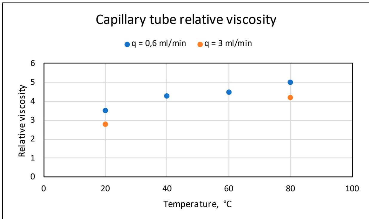
Figure 2 Measured mobility reduction in capillary tube.
