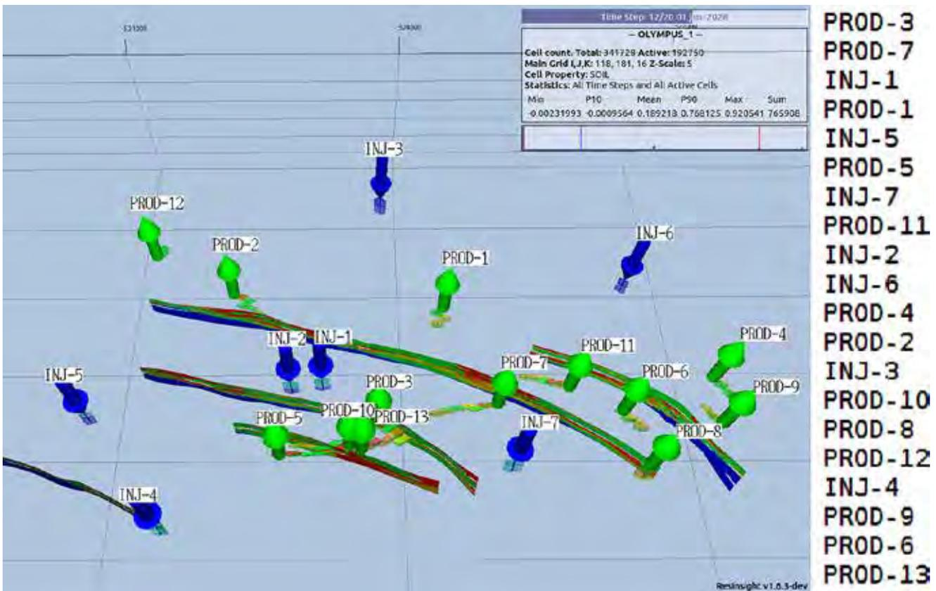
Optimal well locations. The drilling order is provided on the right.
