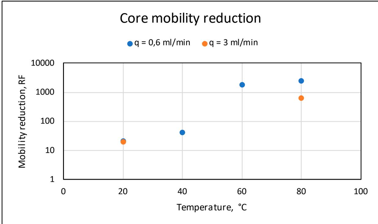
Figure 1 Measured mobility reduction in sand column.
