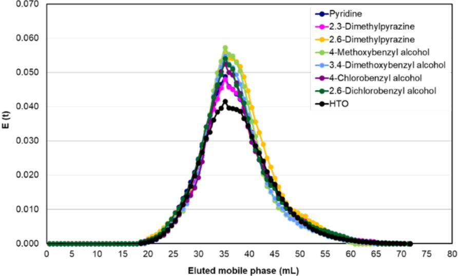
E (t) vs eluted mobile phase in the flooding experiments with a water-saturated chalk core.
