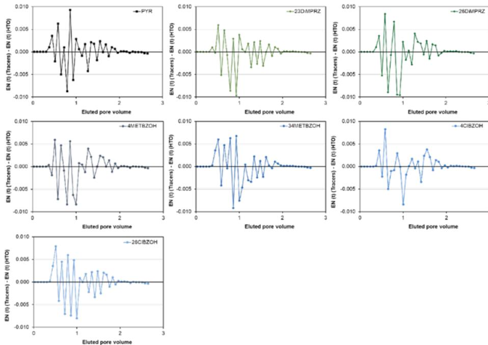
EN (t) of the PITT tracer candidates – EN (t) of HTO vs eluted pore volume in the water saturated sandstone core.
