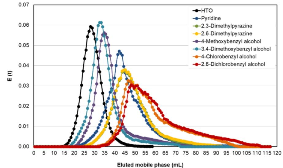
$E(t)$  vs eluted mobile phase in the flooding experiments with the chalk core in  $S_{OR}$  conditions
