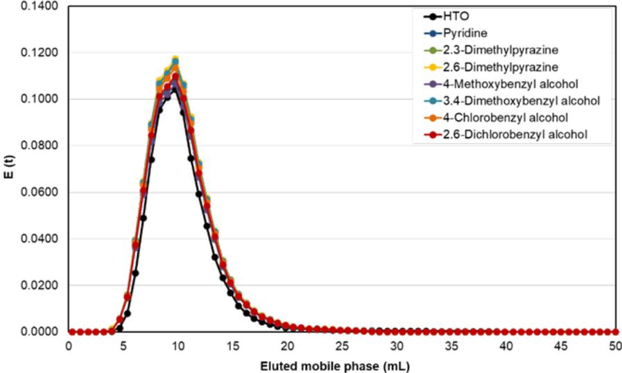
E (t) vs eluted mobile phase in the flooding experiments with a water-saturated sandstone core.
