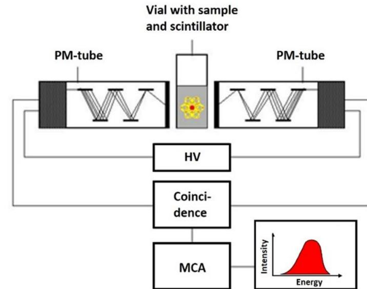
Simplified liquid scintillation counter scheme
