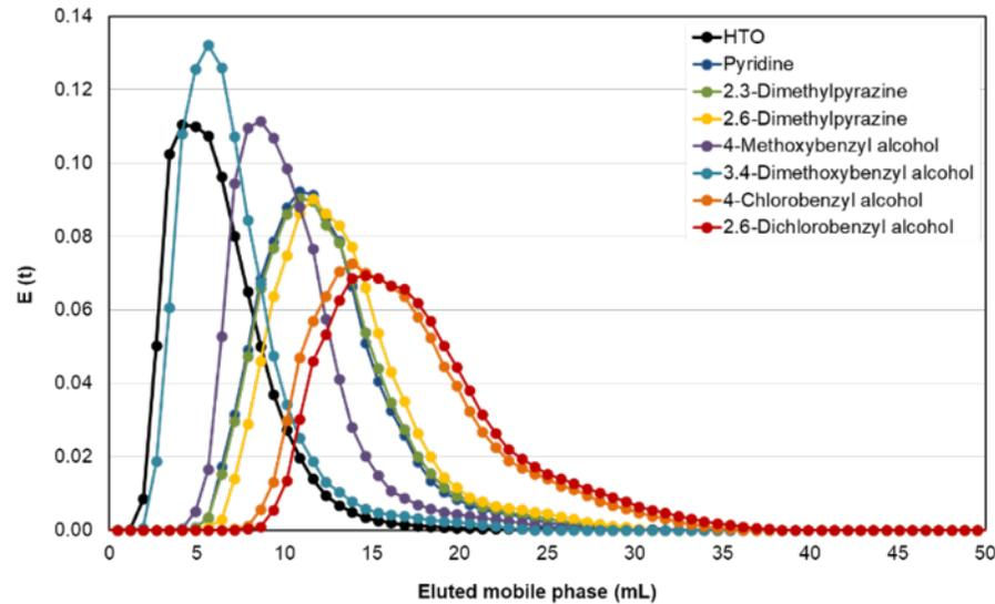
$E(t)$  vs eluted mobile phase in the flooding experiments with the sandstone core in  $S_{OR}$  conditions
