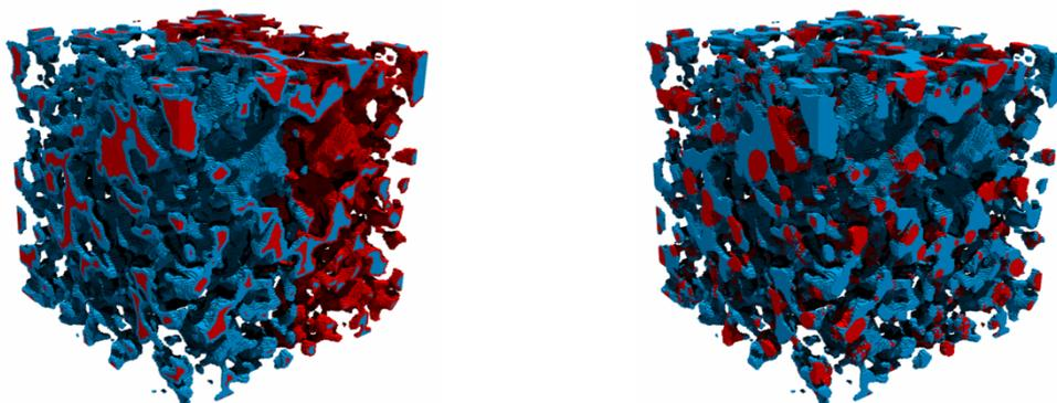
Figure 4: Snapshots from a relative permeability simulation using a water-wet sandstone sample of 200x200x200 voxels. The initial configuration is shown to the left, and the configuration after 1.5 pore volumes is shown to the right. The simulation is executed at the HPC cluster [fram.sigma2.no](http://fram.sigma2.no) hosted at UiT Arctic University of Tromsø.
