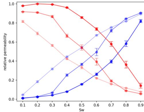
Figure 7: Relative permeability plots (red for oil, blue for water) for the sandstone sample at three different wetting values. Pale colors represent the oil wet sample, intermediate hue colors represent the neutral wet sample, and strong colors represent the water wet sample.
