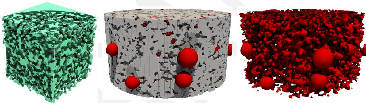
Figure 2: Spontaneous imbibition simulation in a cylindrical Bentheim sandstone sample of 4 mm in diameter with oil shown in red. The left figure shows pore space in green for one quadrant of the sample, the middle figure shows solid space in gray and oil in red after 50 minutes of imbibition, and the right figure shows the internal distribution of oil.
