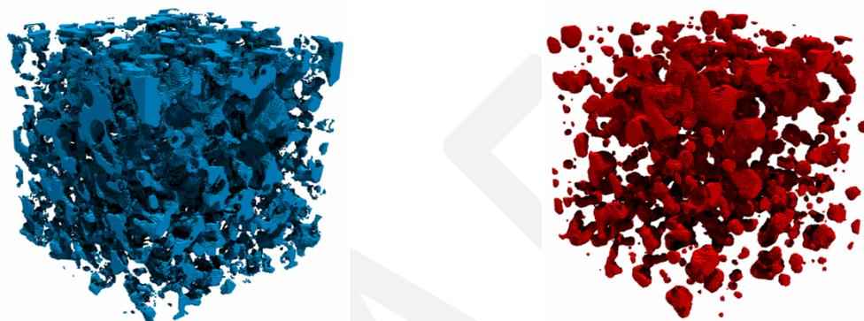
Figure 5: Water- (left) and oil-distribution (right) after 1.5 pore volumes (same as in Figure 1, right)
