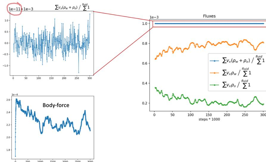
Figure 6: Demonstration of our novel method for constant flux conditions during relative permeability simulations with an accuracy of  $10^{-11}$ . The body-force driving the flow is constantly varying to keep the flux constant.
