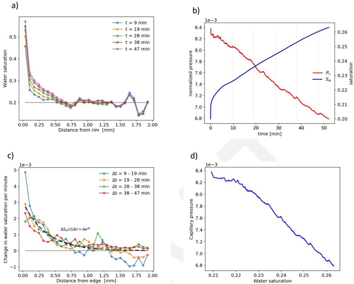
Figure 3: Results of a spontaneous imbibition simulation in a Bentheim sandstone sample 4 mm in diameter; a) shows the radial distribution of water saturation for different times; b) shows the evolution in water saturation together with the capillary pressure (the vertical lines indicate the times in a) and c)); c) shows the change in water saturation for different time-intervals at different radial positions; d) shows the capillary pressure as function of water saturation.
