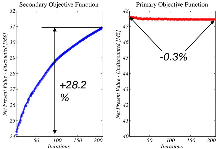
Optimization of secondary objective function - unconstrained
