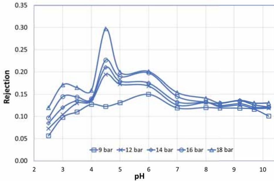
Figure 6. Na<sup>+</sup> rejection with varying pH for ESNA
