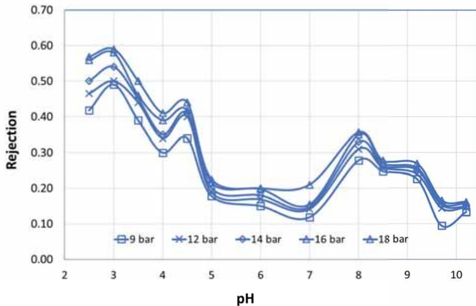
Figure 14.  $\text{Ca}^{2+}$  rejection observed for ESNA at different feed pH
