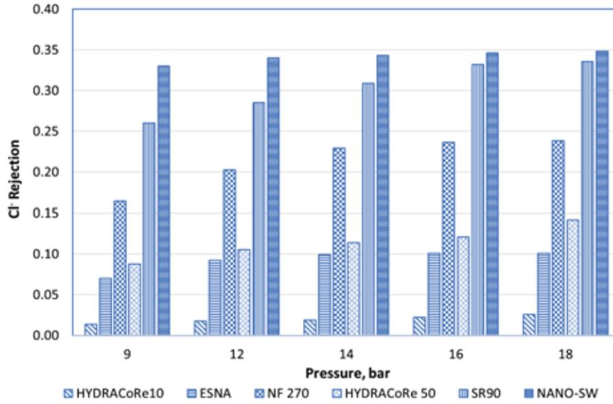
Figure 13. Cl<sup>-</sup> rejection for six NF membranes
