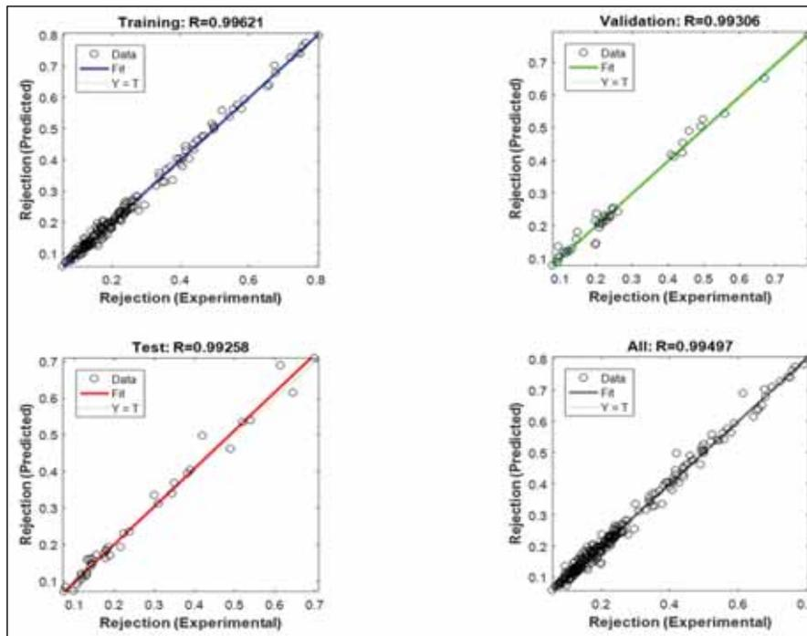
Figure 16. Regression plot between the experimental and predicted rejection values for ESNA with 7 neurons in the hidden layer
