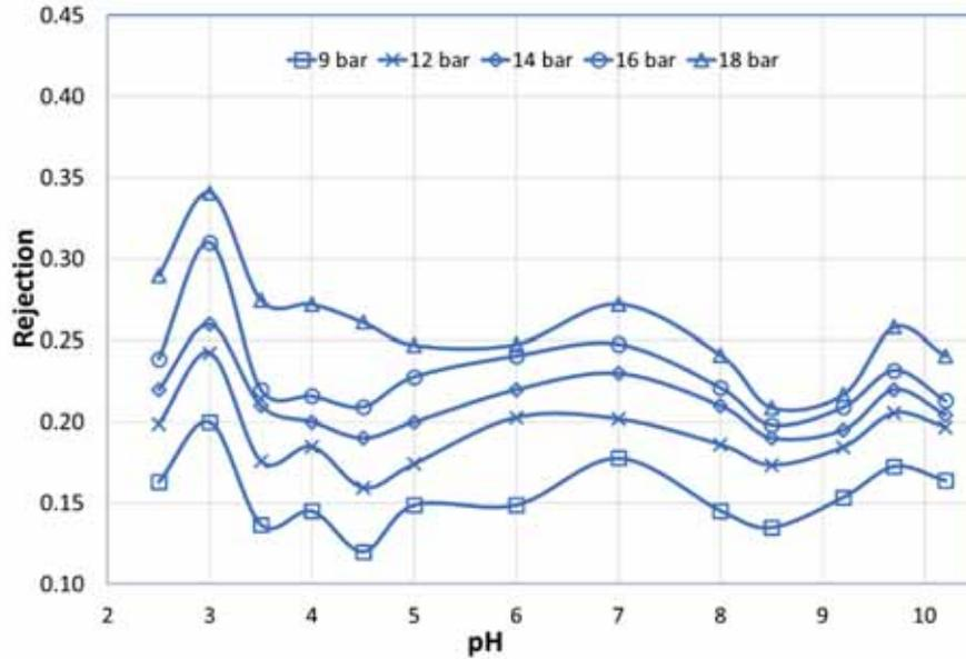
Figure 26. Effect of pH on Na<sup>+</sup> rejection with NF 270
