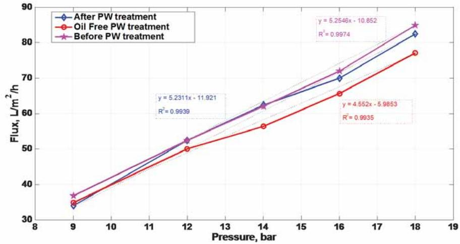
Figure 4. Flux comparison for seawater before and after treating oil-free PW by NF 270-2540
