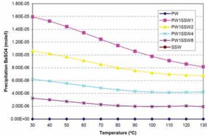
Figure 2. BaSO<sub>4</sub> precipitation versus temperature from a combination of SSW and Tor field PW (Punternold, 2008)
