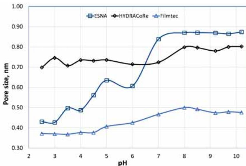
Figure 27. Variations in pore size with feed pH
