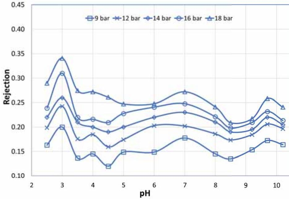
Figure 10. Na<sup>+</sup> rejection at different feed pH for NF 270
