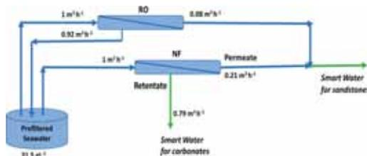
**Figure 13.** Suggested schematic for smart water production in carbonate and sandstone reservoirs.
