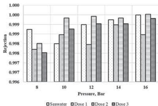
Figure 6.  $\text{SO}_4^{2-}$  rejection at three added doses of sulfate in seawater.
