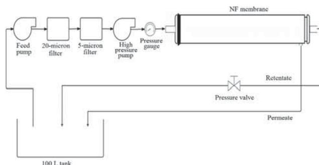
Figure 1. Schematic of the NF membrane pilot unit used for experiments.
