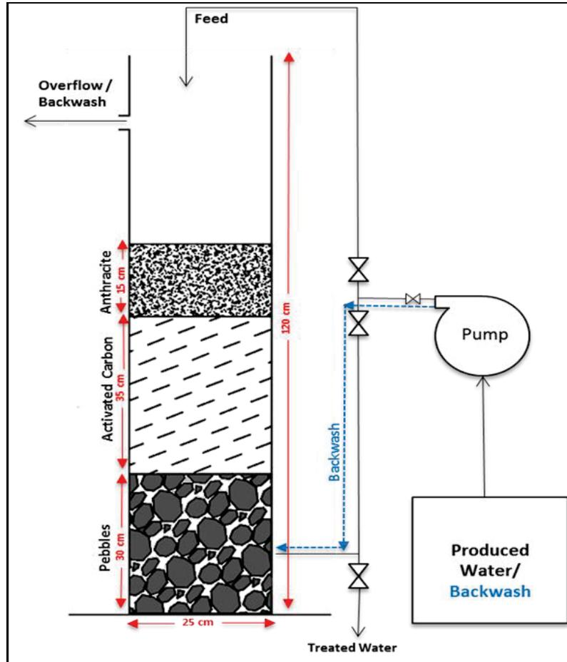
Figure 11. Schematic of the lab-scale media filtration unit
