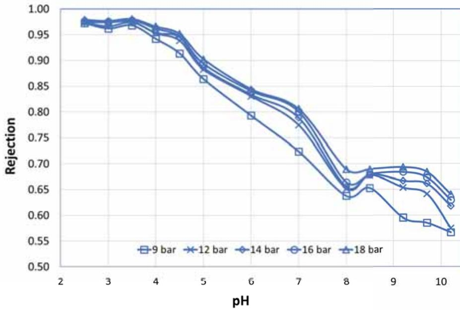
Figure 13. Mg<sup>2+</sup> rejection at different feed pH for NF 270
