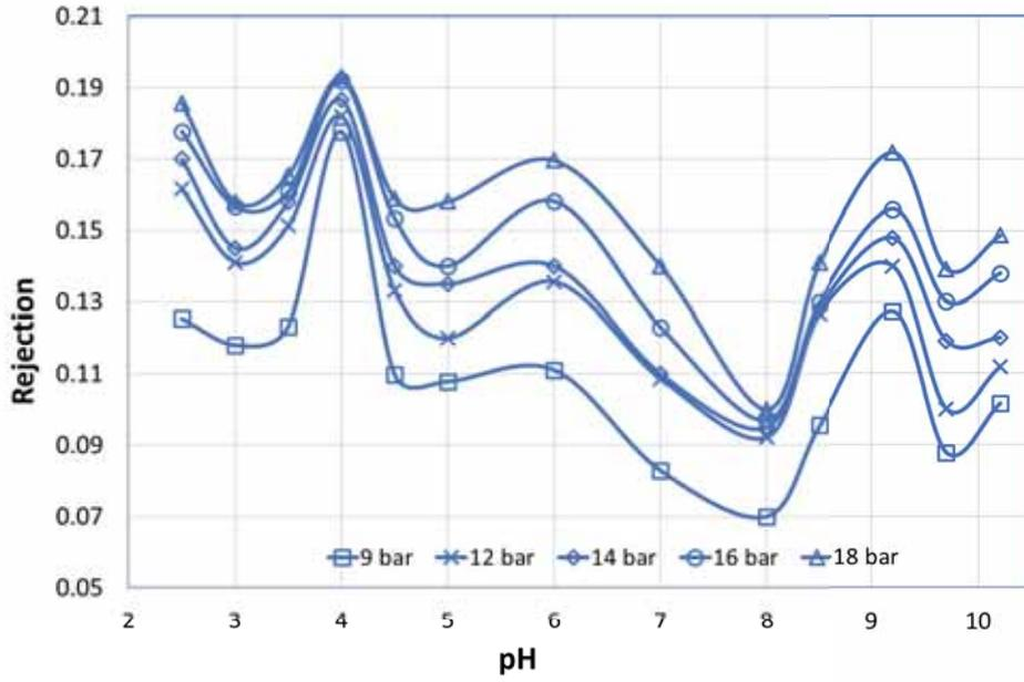
Figure 7. Cl<sup>-</sup> rejection for HYDRACoRe at different feed pH
