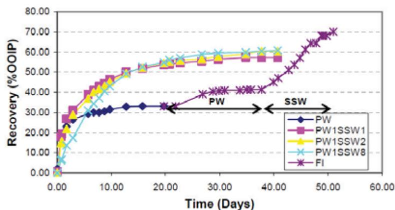
**Figure 1. Spontaneous imbibition of mixtures of PW and SSW into chalk cores at 110°C saturated with a crude oil of acid number = 0.70 mg KOH/g oil (Puntervold, 2008)**
