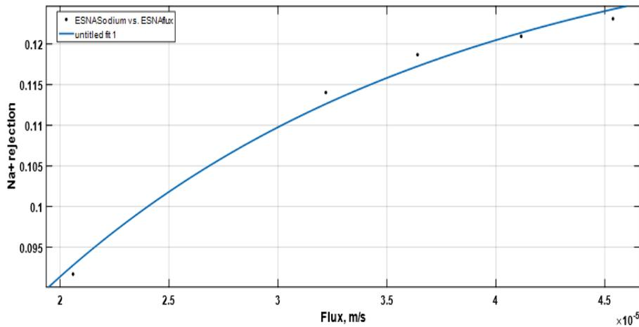
Figure 29. Rejection versus flux for  $\text{Na}^+$  for ESNA
