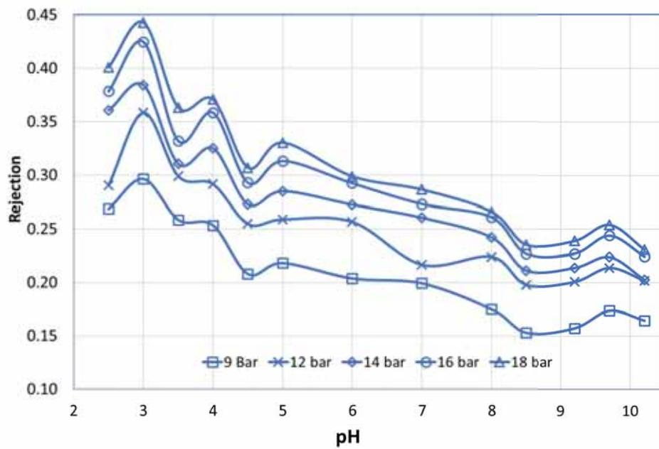
Figure 9. Cl<sup>-</sup> rejection at different feed pH for NF 270
