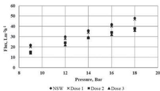
Figure 9. Comparing flux versus pressure for seawater and seawater spiked with  $\text{MgCl}_2$ .
