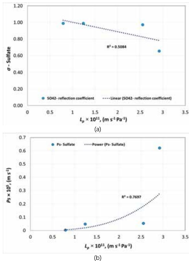
Figure 5. Pure water permeability versus (a) reflection coefficient and (b) solute permeability of sulfate.
