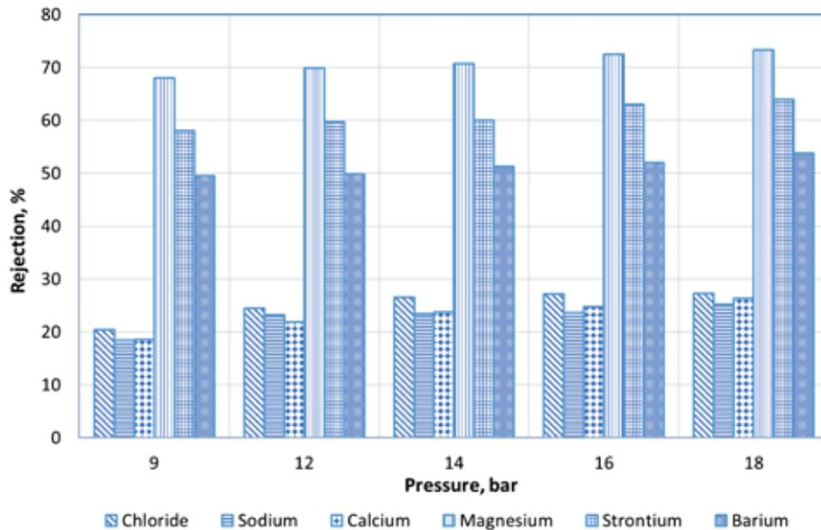
Figure 19. Rejection of  $Ba^{2+}$  and  $Sr^{2+}$  with NANO-SW
