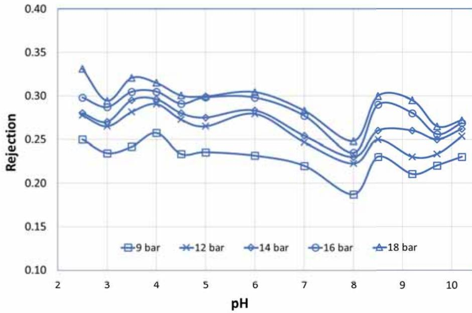
Figure 12. Mg<sup>2+</sup> rejection at different feed pH for HYDRACoRe
