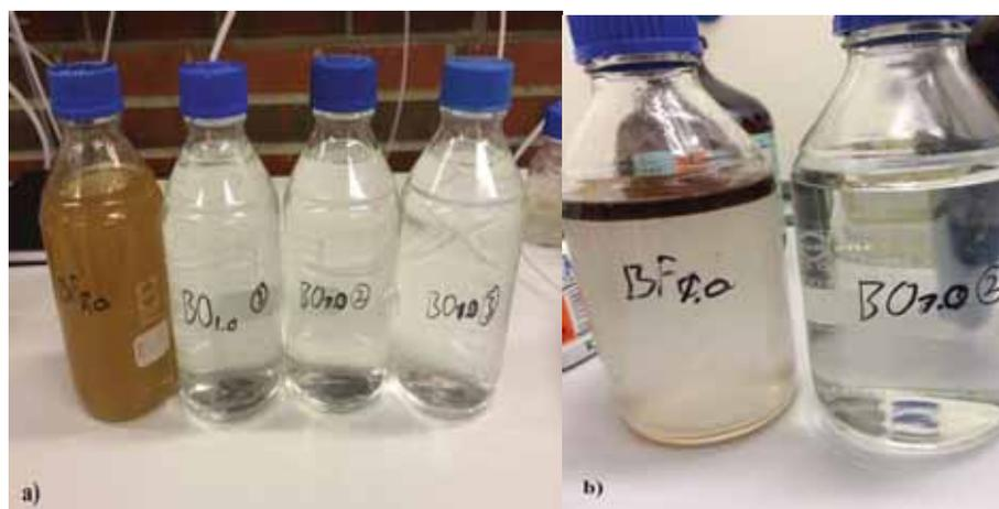
Figure 18. Comparison of influent and effluent samples a) before extraction b) after extraction
