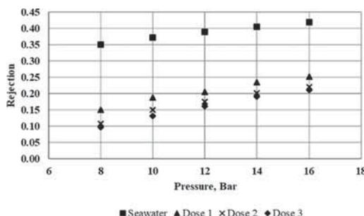
Figure 5.  $\text{Cl}^-$  rejection versus pressure with an increase in the  $\text{Na}_2\text{SO}_4$  concentration.
