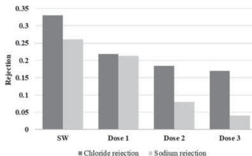
**Figure 12.** Rejection of  $Cl^-$  and  $Na^+$  at 8 bar with different  $Ca^{2+}$  concentrations.
