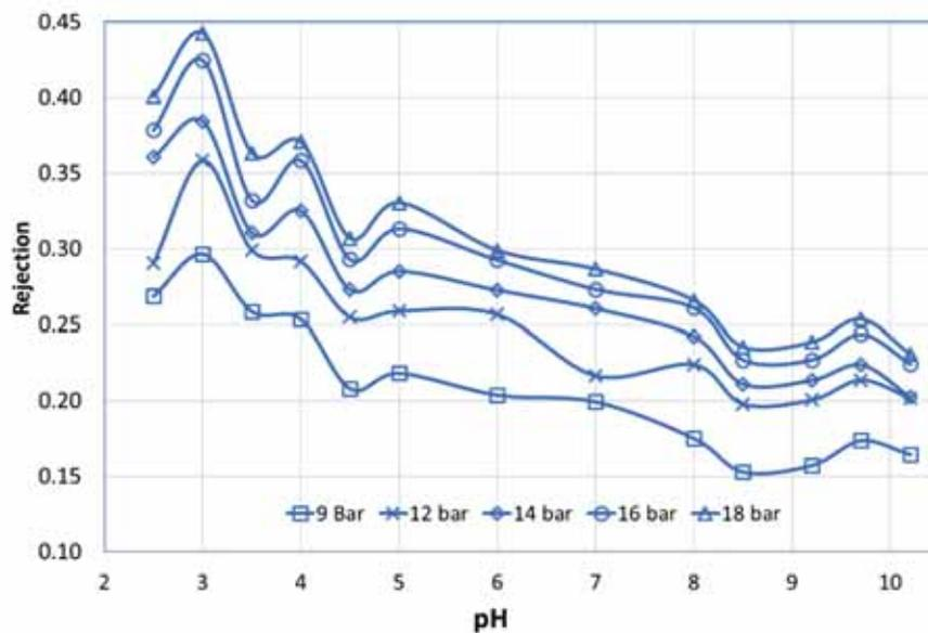
Figure 25. Effect of pH on  $\text{Cl}^-$  rejection for NF 270
