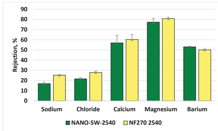
Figure 5. Rejection % by NANO-SW-2540 and NF270-2540 at 18 bar
