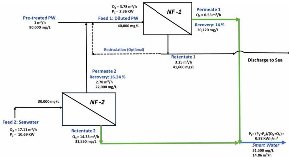
Figure 7. Suggested process schematic for Smart Water production
