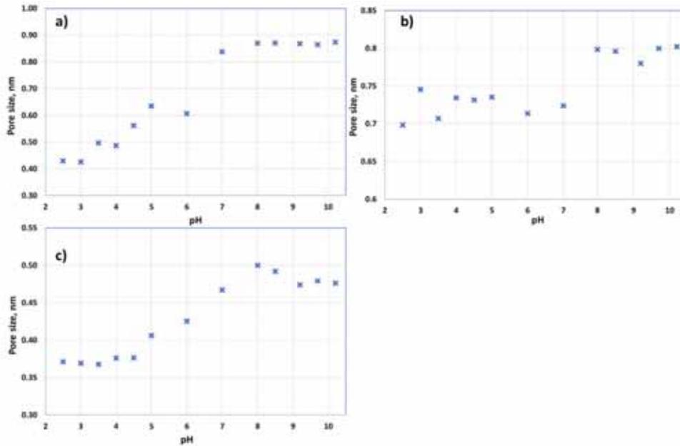
Figure 15. Variations in  $r_p$  with pH on a) ESNA b) HYDRACoRe c) NF 270
