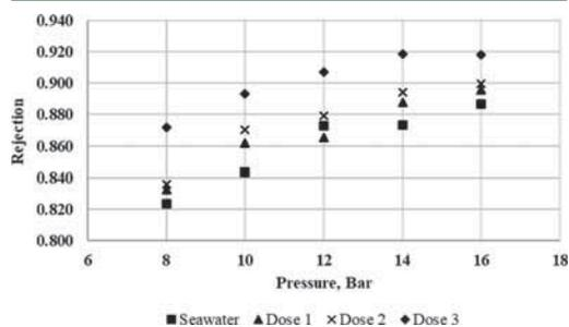
Figure 7.  $\text{Mg}^{2+}$  rejection with increased  $\text{SO}_4^{2-}$  concentrations.
