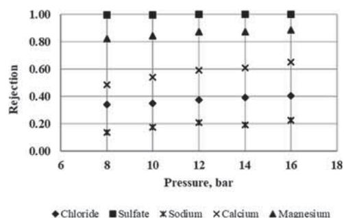
Figure 3. Ion rejection with NANO-SW-2540.
