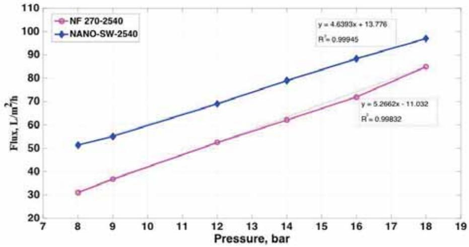
Figure 6. Flux versus pressure for NF270-2540 and NANO-SW-2540
