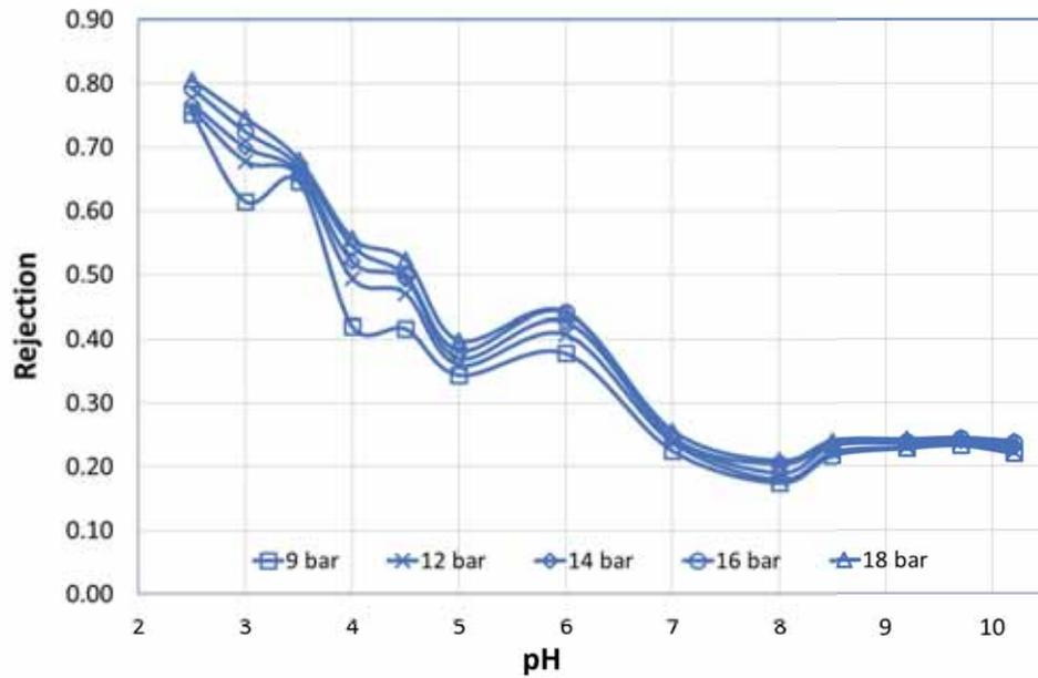
Figure 11. Mg<sup>2+</sup> rejection at different feed pH for ESNA
