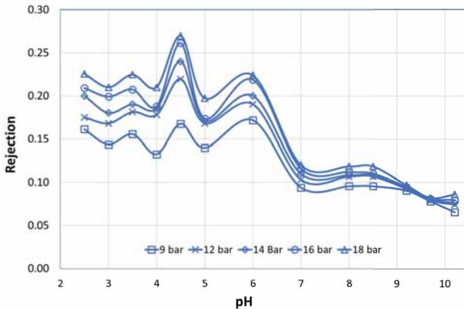
Figure 5.  $\text{Cl}^-$  rejection for ESNA
