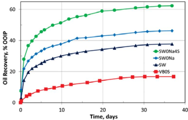
Figure 9. Spontaneous imbibition of brines into oil saturated chalk cores at 90 °C with VB (FW), seawater (SW), and modified seawater (SW0NaCl, and SW0NaCl- 4 × SO<sub>4</sub><sup>2-</sup>) [32]
