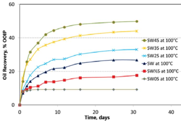
Figure 6. Spontaneous imbibition of brines with varying  $\text{SO}_4^{2-}$  concentrations into fractional intermediate wetted chalk cores [30]
