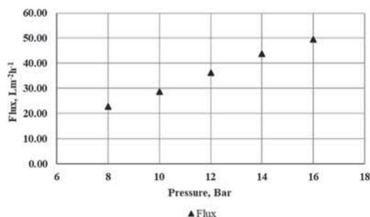
Figure 2. Flux versus pressure with seawater as feed.
