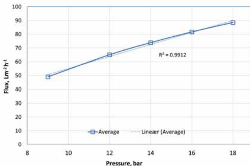
Figure 20. Flux versus pressure with Ba<sup>2+</sup> and Sr<sup>2+</sup> in the feed
