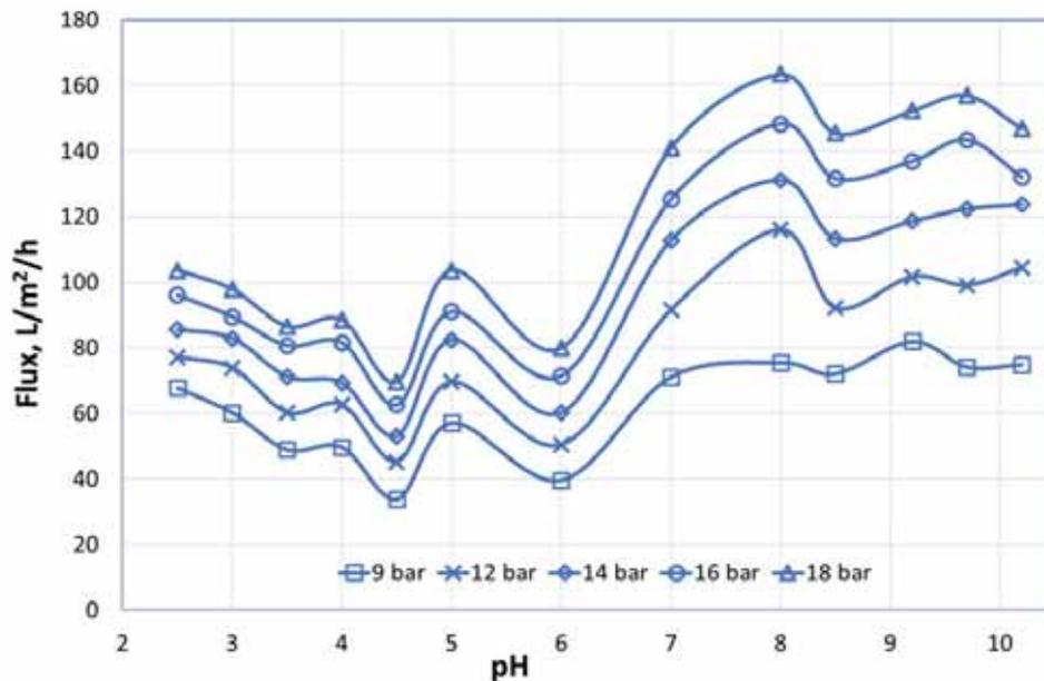
Figure 2. Flux versus pressure for ESNA at different pH
