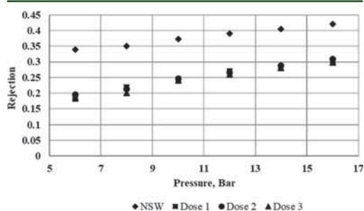
**Figure 11.** Rejection of  $Cl^-$  with an increased  $Mg^{2+}$  concentration in the bulk phase.
