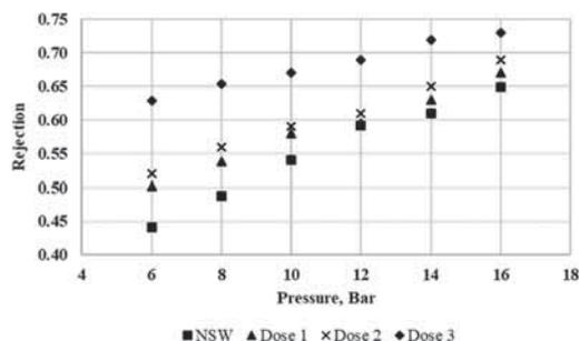
Figure 8. Observed  $\text{Ca}^{2+}$  rejection with a corresponding increase in the  $\text{Na}^+$  concentration.
