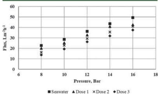
Figure 4. Flux versus pressure for seawater and seawater spiked with  $\text{Na}_2\text{SO}_4$ .
