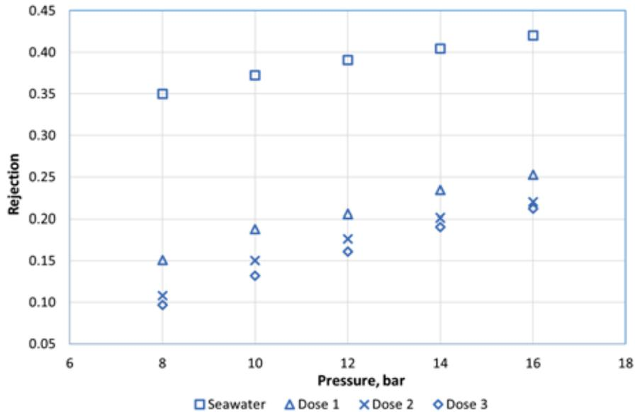
Figure 17. Cl<sup>-</sup> rejection with increased SO<sub>4</sub><sup>2-</sup> concentration
