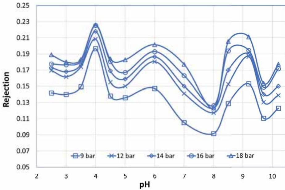
Figure 8. Na<sup>+</sup> rejection at different feed pH for HYDRACoRe
