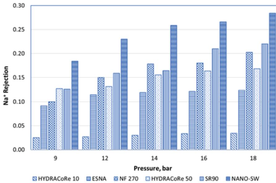
Figure 14. Na<sup>+</sup> rejection for six NF membranes
