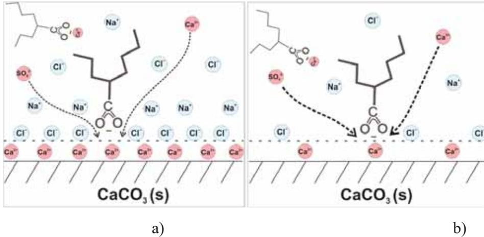
Figure 4. Schematic of mechanisms for wettability alteration in carbonates a) Mechanisms when monovalent ions are present b) Mechanisms with increased  $\text{Ca}^{2+}$  and  $\text{SO}_4^{2-}$  and decreased  $\text{Na}^+$  and  $\text{Cl}^-$  concentrations [28].
