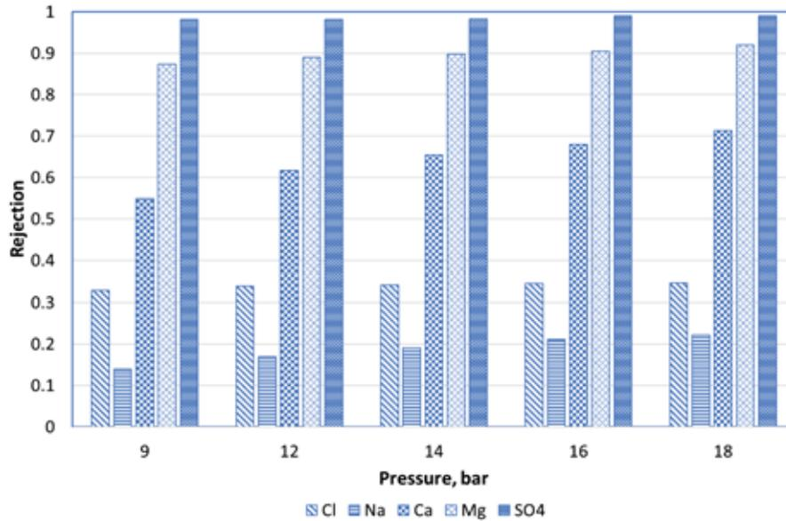
Figure 12. Ion rejection with increasing pressure with NANO-SW
