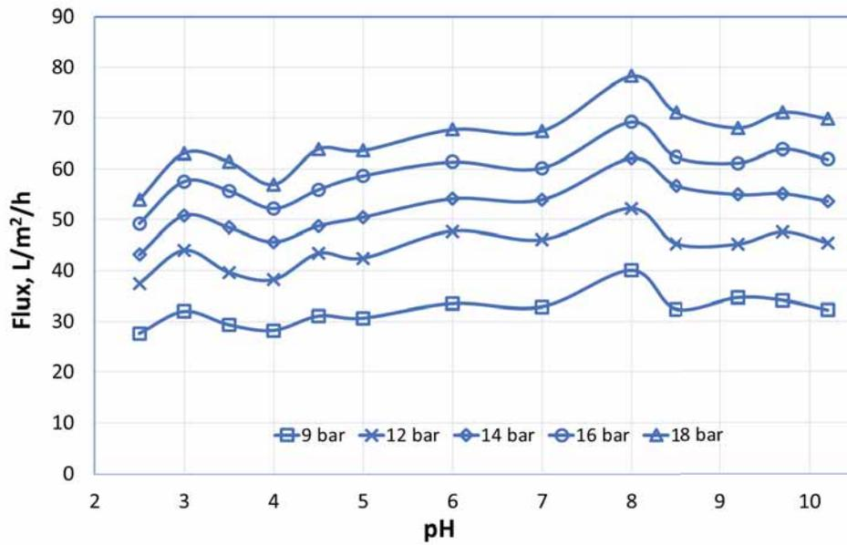
Figure 3. Flux versus pressure for HYDRACoRe with varying pH
