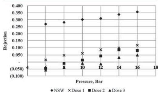
Figure 10. Negative rejection of  $\text{Na}^+$  with increased  $\text{Mg}^{2+}$  in the bulk phase.
