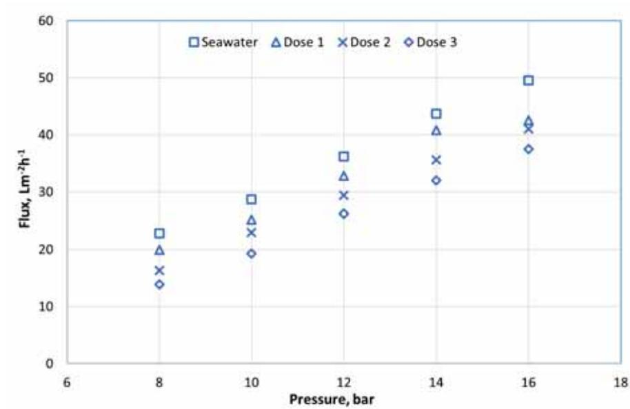
Figure 16. Flux variations with increased  $\text{SO}_4^{2-}$  concentrations in the feed
