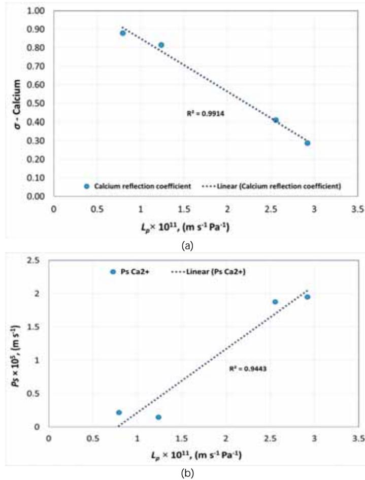
Figure 6. Pure water permeability versus (a) reflection coefficient and (b) solute permeability of calcium.
