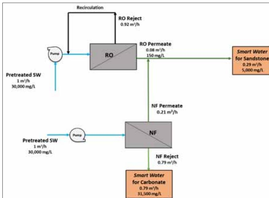
Figure 31. Schematic for smart water production from seawater
