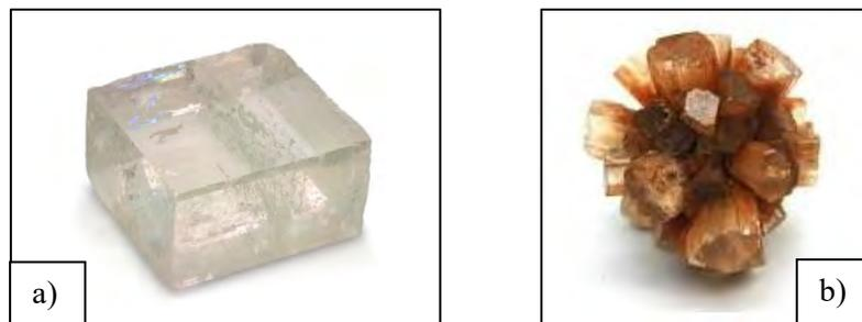
Figure 37 – Calcite (a) and aragonite (b) crystals.
