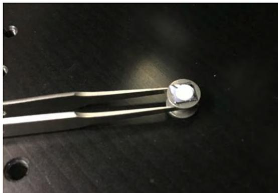
Figure 52 - The best way to study chalk samples by TERS is to drill out little disks from cores thin section and carefully polish them.
