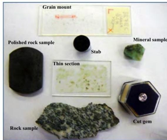
Figure 31 - Raman spectroscopy does not need sample preparation and can be performed directly on minerals, thin sections or cut gems.
