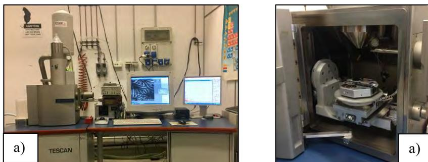
Figure 60 - The EDS spectrometer coupled to SEM (Scanning Electron Microscope) present at the Milano-Bicocca University (a) and its sample holder (b).
