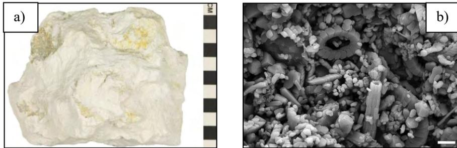
Figure 41 – a) An example of a chalk rock sample , centimetric scale bar . b) A SEM micrograph of Liège chalk before flooding . Scale bar: 2 micron. From Wang et al. 2016.
