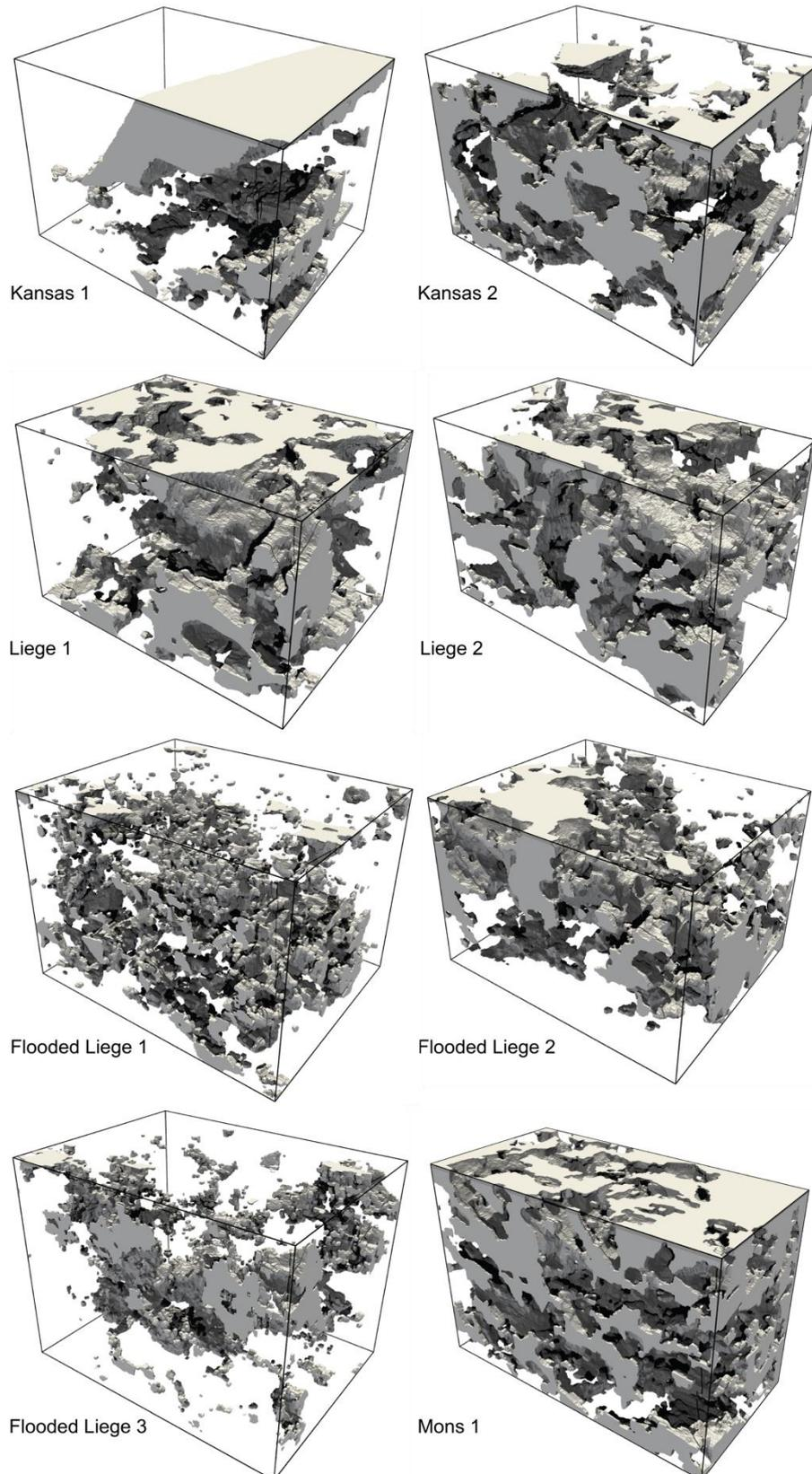
Figure 4: Three-dimensional representations of the pore space of eight chalk samples. Porosity, permeability (flow from right to left), and size of the samples are listed in Table 1. A FIB-SEM image from each of the samples is shown in Figure 2.
