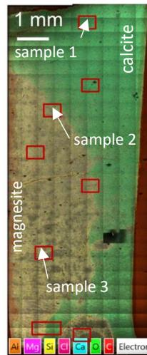
*Figure 1: Map of the flooded Liege sample where a magnesite dominated region in yellow meets a calcite dominated region in green at a sharp interface. The locations of the pore geometries obtained from this core sample subset is indicated as red squares. Sample 1 represents the unaltered calcite dominated part of the core, sample 2 is obtained at the interface between the two regions, while sample 3 represents the altered magnesite dominated region.*
